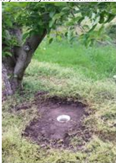
Fig. 1. Soil trap type Barber
